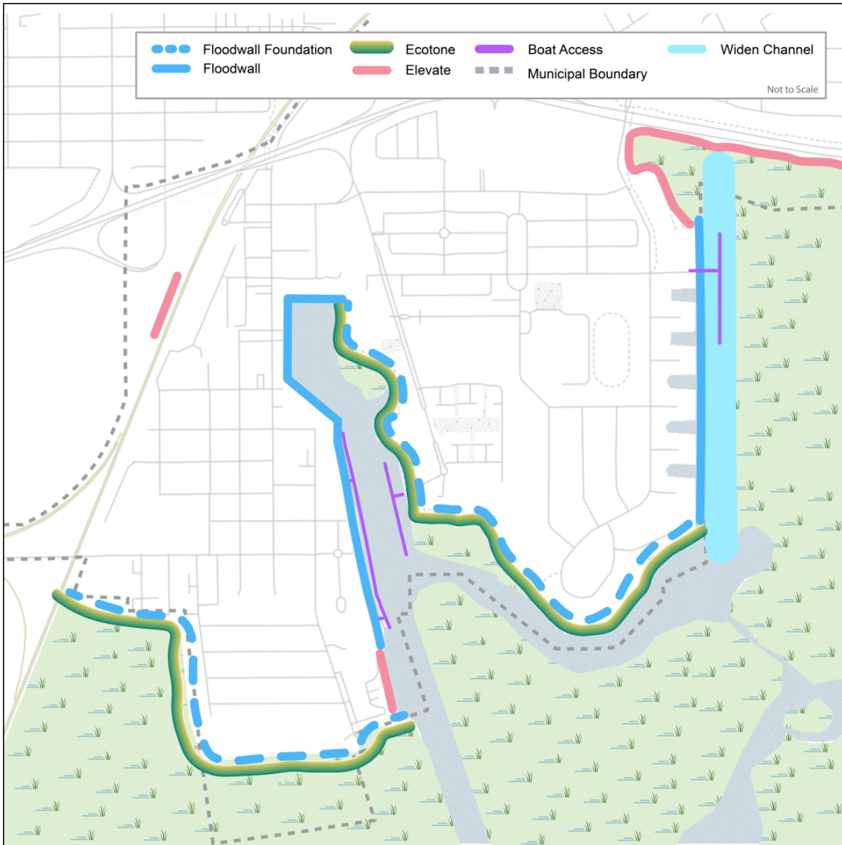
Mid-term adaptation scenario, assuming 52 inches total water level over recent levels, from the Suisun City case study showing waterfront protection options (including an “ecotone” or “horizontal” levee).
